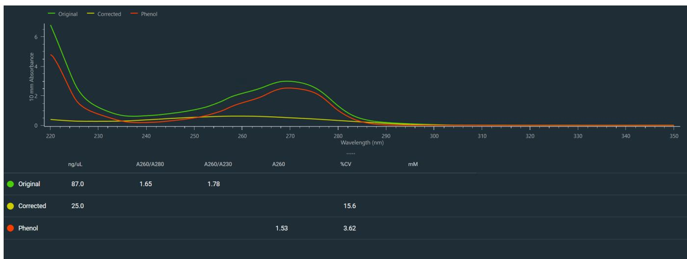
Figure 1: RNA spectra with phenol contamination, identified by Acclaro technology. The NanoDrop One/One<sup>c</sup> software reports the corrected RNA concentration and spectrum in yellow.
