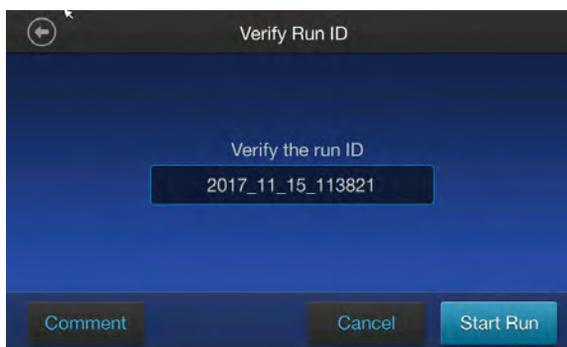
4. (Optional) In the **Run Parameters** screen, press the field under **Verify the run ID**, then enter the applicable information in the **Enter the Run ID** screen.
