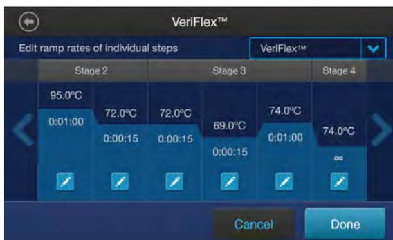
3. In the **Edit VeriFlex™** screen, adjust the temperature range across the block for the selected steps.
