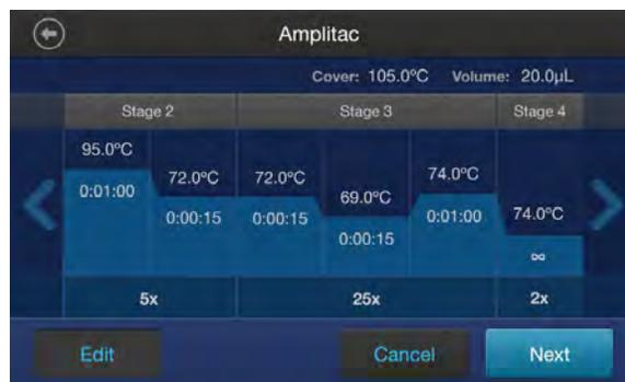
2. Edit any of the parameters that are surrounded by black fields indicating that they are editable (temperature, time, heated cover, number of cycles, and volume).
