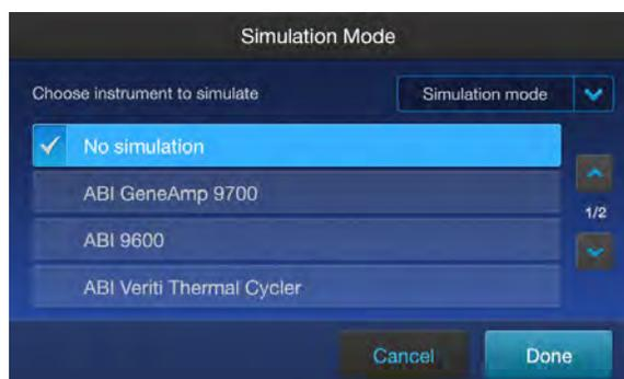
**Note:** Press **No Simulation** to run the instrument in the default mode.
